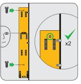
Securely attach the mounting plate vertically to the wall with the strap fitting at eye-level.
