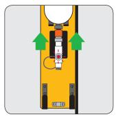
Using the quick-connect fitting attach the purity light to the bottom of the cartridge.
