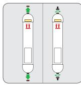
Remove the red caps from the cartridge and thread on the 2 male quick-connect fittings.
