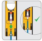
Attach the blue Output Hose to the purity light by using the threaded connection.
