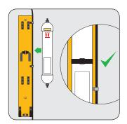
Re-attach the cartridge to the mounting plate using the strap. Ensure arrows are pointing up.
