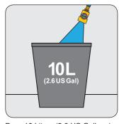
Pass 10 Litres (2.6 US Gallons) of water through the system into a bucket.
