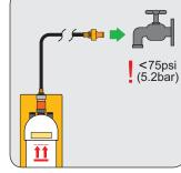
Connect the free end of the black inlet hose to the water supply.
